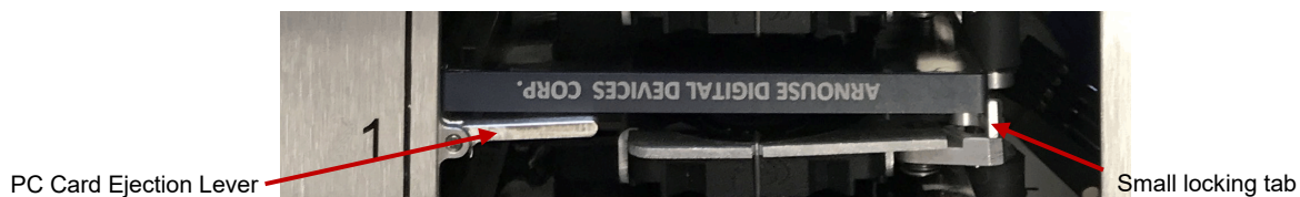
Figure 9- PC Card Fully Inserted and locked
