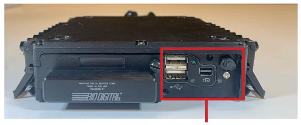
Remove the front right cover by loosening the two bolts on it. Once the cover is removed it will expose (2) USB 2.0 ports and a MiniDP video port.
