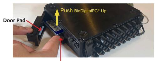
You must push the BioDigitalPC® up as you close the door so that the door pad shown above won't interfere with door's normal operation.
