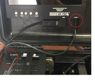
**◆** CONNECT THE 12VDC DISPLAY CABLE
