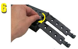
Once the BiodigitalPC® is fully docked, close the door and lock it by turning the screw with D-ring clockwise.
