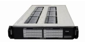
out of rack placement 36" to expose entire shelf. The SR-60 can be operated hot or cold aisle. The SR-60 is composed of 6, SR-10 modules, each module comes with 10 BioDigitalPC® card slots (cards sold separately), and (3) Gigabit NICs. All 30 Gigabit NICs are then connected to a shared managed ethernet switch with 2 SFP+ 10 Gb interconnects and an auxiliary 1 Gb connection.
