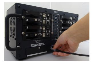
Plug in the supplied AC to DC power supply into the 12-36 VDC power connector.
