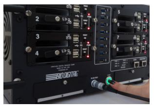
To power down the MDC-8, press the PWR button for 3 seconds.
