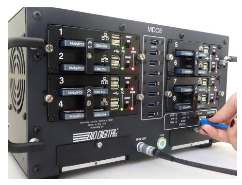
Located on the front of the MDC-8 you will find a 1Gb WAN port and 1Gb DMZ/WAN port. These allow for a dual WAN scenario. You may also configure the DMZ/WAN port as a DMZ for public facing services. The MDC-8 also contains 6 internal LAN ports. These LAN ports can be routed to the front panel connectors if requested or needed,
