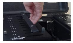
Prior to inserting the server card(s), you must remove the cover to the card holder.
